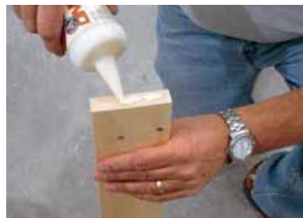
Fig. 2 ASSEMBLE THE L. It's a good idea to use yellow carpenter's glue as well as drywall screws to assemble the supports. To ensure the wood doesn't split when driving in the screws drill a couple of pilot holes with a small drill bit.
