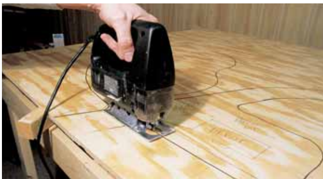
Fig. 3 CUTTING. Use a saber saw (jigsaw) to make the cuts. To avoid cutting through your benchwork, raise the plywood above the benchwork with scrap 2 x 2s or 2 x 4s.
