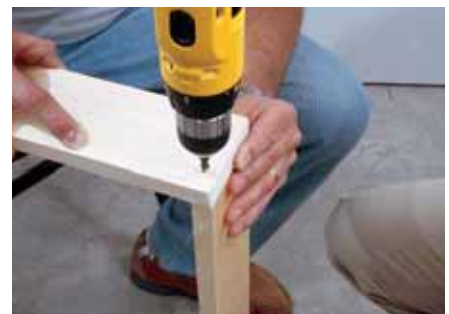
Fig. 2 ASSEMBLE THE L. It's a good idea to use yellow carpenter's glue as well as drywall screws to assemble the supports. To ensure the wood doesn't split when driving in the screws drill a couple of pilot holes with a small drill bit.
