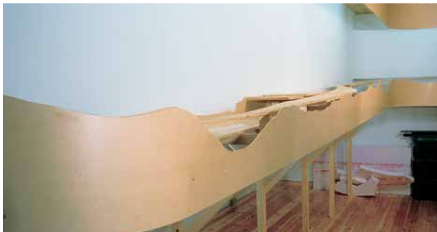
Fig. 6 Completing the frame. Pelle used a jigsaw to cut the fascia on the pencil lines representing the scenic contours. With the valance, lighting, benchwork, and fascia in place, Pelle could finally move on to the modeling part of the hobby.
