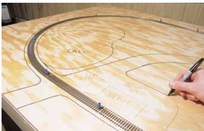
Fig. 2 SKETCH DETAILS. Along with track center lines you'll need to outline details such as roads, lakes, rivers, parking lots, and structures. Use a marker to draw the cutting lines.
