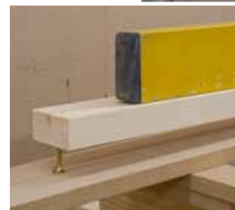
I cut out the subroadbed from 1/2" MDF. The grades on my layout are kept around 2.0–2.2 percent. I placed wood blocks under the subroadbed to build up the grades. I used a homemade tool to measure the exact grade. The tool consists of a 1-meter-long board with a screw attached to one end and a carpenter's level placed on top of it. How long the screw sticks out defines the steepness of the grade. If it sticks out 2cm, the grade is 2 percent on a level board.
