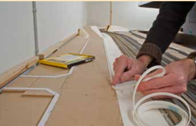
3. On the other side of the road, I applied Woodland Scenics Paving Tape along the outside edge of the street. Paving Tape is a foam tape approximately .040" thick.
