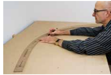
I drew the center lines for the track on the subroadbed at the Daneville area, utilizing my homemade "curve-with-easement ruler" that has a 33" radius curve on the outside and a 31" radius curve on the inside.
