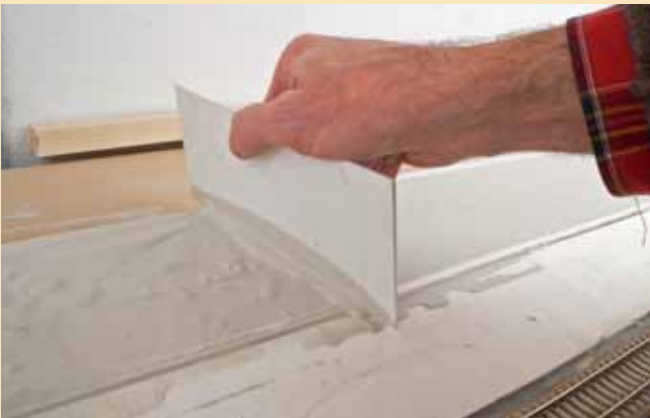
5. I spread the plaster evenly with a piece of styrene. After a few minutes, when the plaster set, I applied a thinner second layer of Smooth-It on top of the first.
