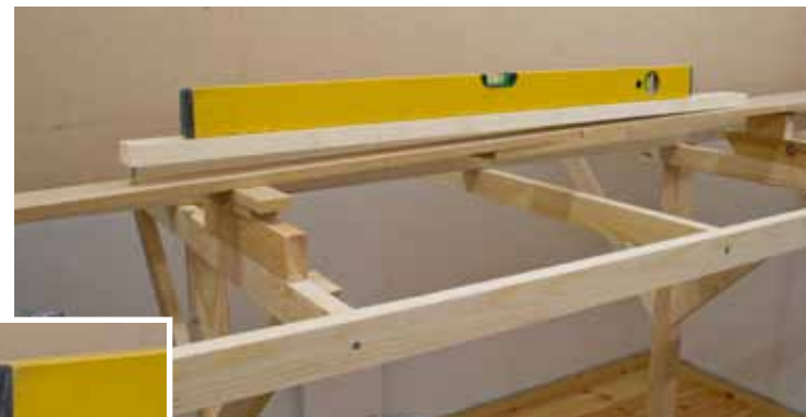
I cut out the subroadbed from 1/2" MDF. The grades on my layout are kept around 2.0–2.2 percent. I placed wood blocks under the subroadbed to build up the grades. I used a homemade tool to measure the exact grade. The tool consists of a 1-meter-long board with a screw attached to one end and a carpenter's level placed on top of it. How long the screw sticks out defines the steepness of the grade. If it sticks out 2cm, the grade is 2 percent on a level board.
