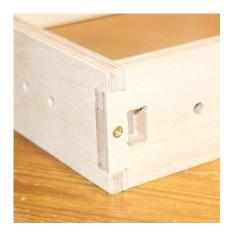
Disassemble the frame, glue all joints and reassemble.
