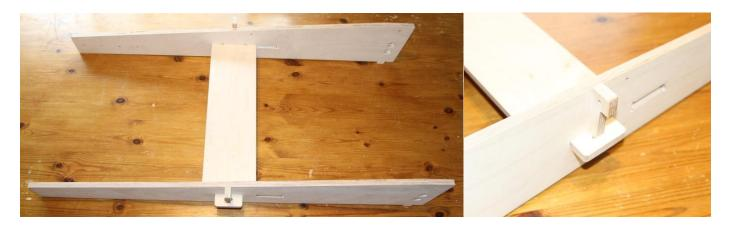
The leg assembly is fitted to the baseboard simply by slotting the locating pegs into the rectangular holes in the end and then fitting the bolts as below.
