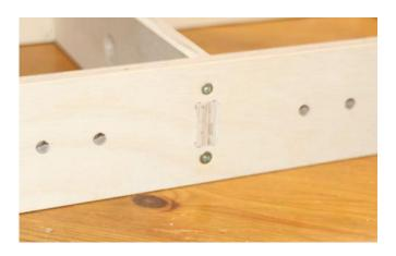
When nailing the tops to the centre 12mm (1/2") wide brace as shown below, angle the nails towards the centre of the brace so they do not come through the sides.
