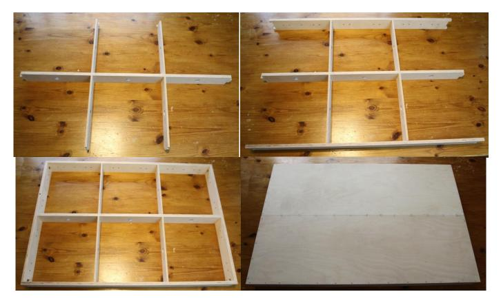
Assembly is similar to the narrower baseboards with the addition of two extra screws in each end as below:
