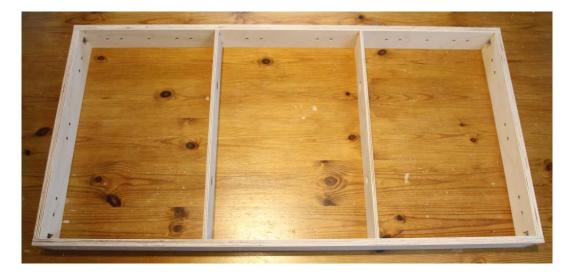
Assemble the frame WITHOUT GLUE to check it fits perfectly. Fit the corner screws as shown below:
