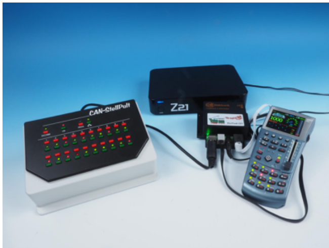
It can also be used as a control panel in a pure CAN-digital-Bahn system structure...
